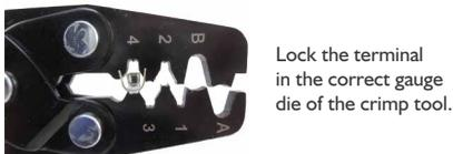
Note: if the terminal crimp tabs are not straight enough the crimper may not crimp them correctly to the cable. Follow Step 6b to straighten the tabs before crimping.
